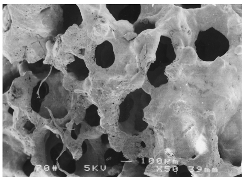
Figure 13 SEM morphology of porous HA from foam of YG-70.
